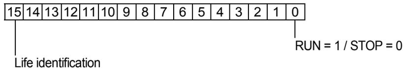
**Error word for USTACK errors of the PLC at DPRAM offset 1042<sub>H</sub>**
