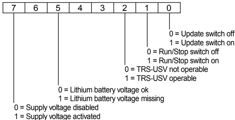
**PB1: Low byte diagnosis register 1 of the lightbus master component**
