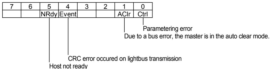
**PB1: High byte diagnosis register 1 of the lightbus master component**
