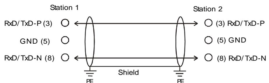
In systems with more than two stations all stations are wired parallel. To be able to connect the cable without interrupt, two cables must be wired into one connector. 9-pole D-sub connectors with switchable termination resistances which ensure an easy cable connection can be ordered from TRS.
