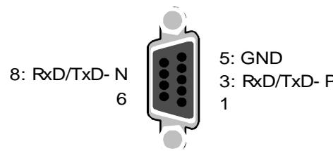
With the BK8000 bus couplers a linear bus can be built up. To prevent reflections during the data transfer it is necessary to terminate the line ends of the bus cable with resistances (120 Ω).
