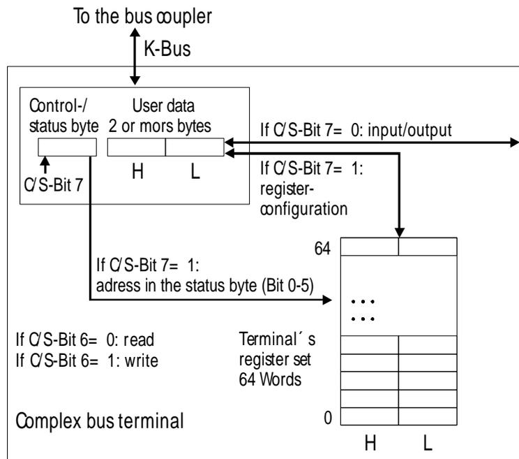
The control or status byte occupies the lowest address of a logical channel. The corresponding register values are located in the following 2 data bytes. (The BK2000 is an exception to this rule: here, an unused data byte is inserted after the control or status byte, thus setting the register value to a word limit.)
