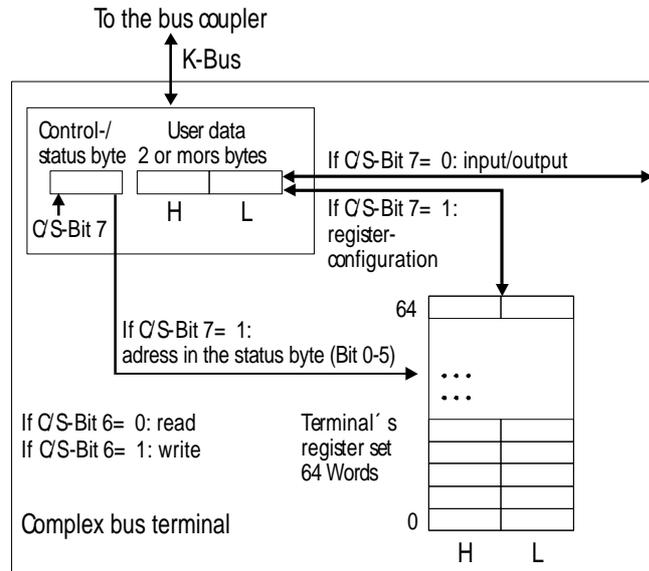
The control or status byte occupies the lowest address of a logical channel. The corresponding register values are located in the following 2 data bytes. (The BK2000 is an exception to this rule: here, an unused data byte is inserted after the control or status byte, thus setting the register value to a word limit.)
