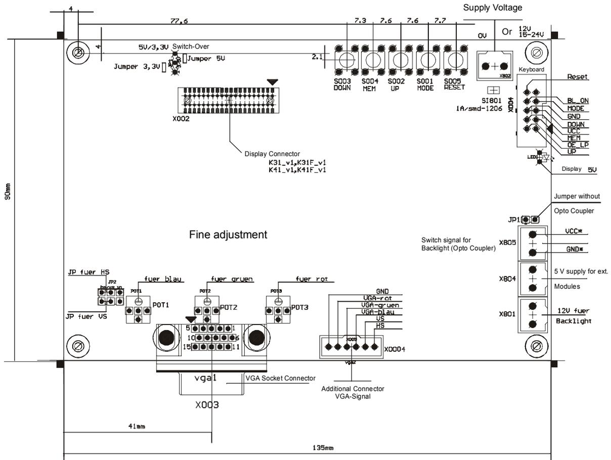
Figure 1: position of the connectors
